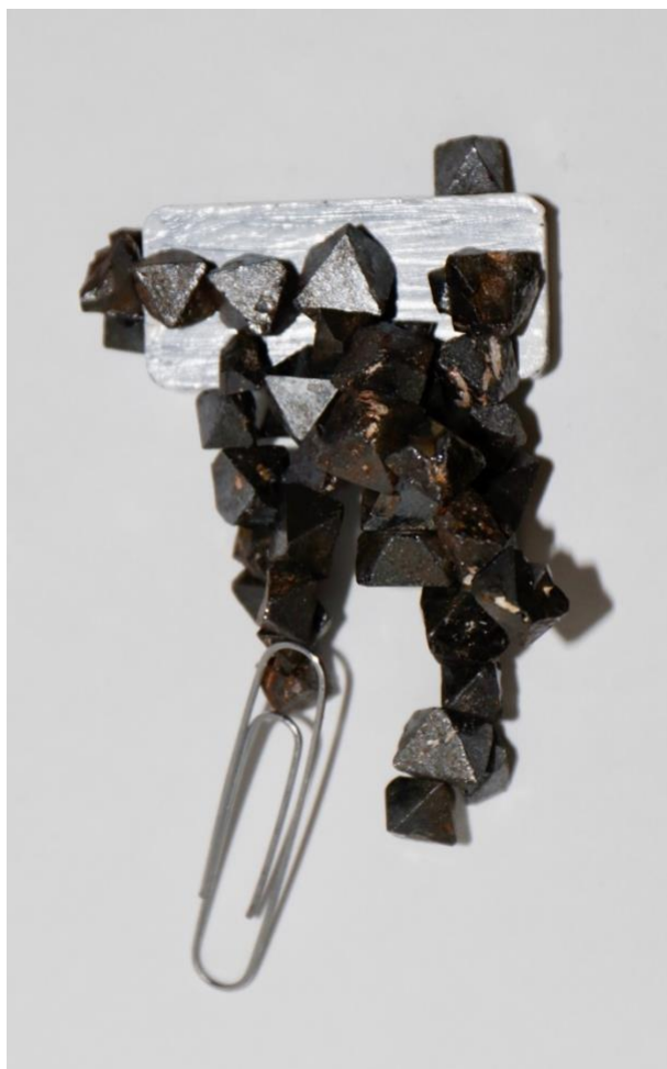
IMAGE 3: This photo demonstrates two properties of Magnetite. One, Magnetite is strongly attracted to magnetic fields. Note the Magnetite crystals clinging to the magnet. Two, Magnetite is one of the few minerals that can become permanently magnetized. Notice how some Magnetite crystals are hanging from other crystals. Also note the paperclip attracted to a crystal. Photo by Tracie J.
