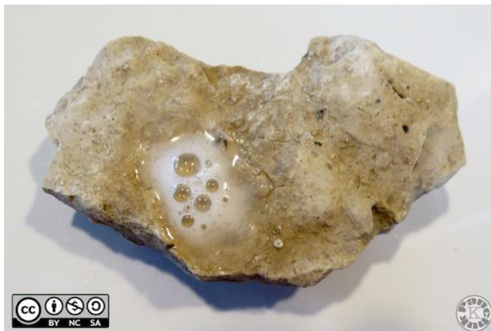
MAGE 1: A piece of Limestone showing the characteristic effervescence (bubbling) result when tested by acid. Source: Karla Panchuk (2020) CC BY-NC-SA 4.0.
