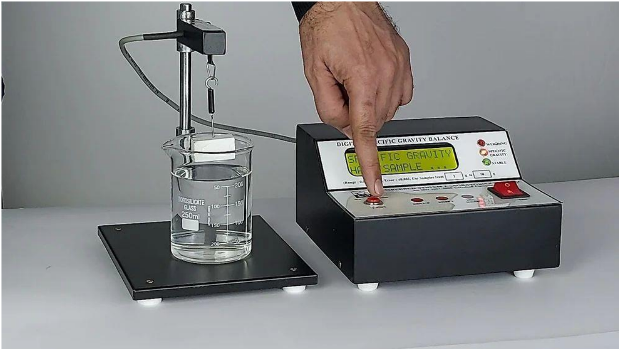
IMAGE 2: Historically there was an instrument, the Jolly Balance, used to calculate specific gravity. Today's technology makes it easier and more accurate. Note the set-up above.
