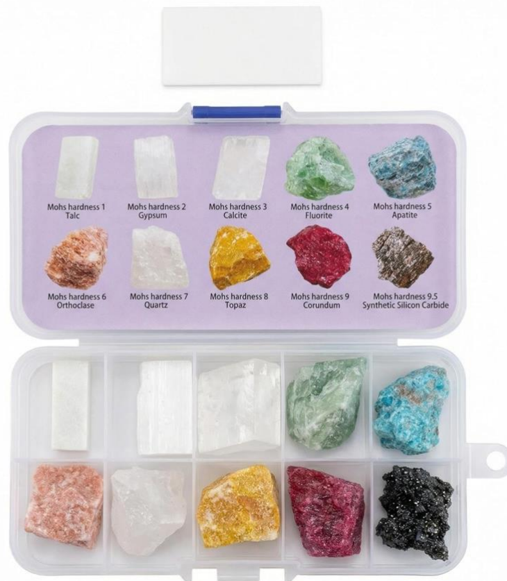
IMAGE 1: Here is a nice example of a set of reference minerals that can be used to test other minerals. It would be easy to make your own.
