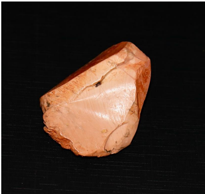
Image 17: An example of Kaolinite with orangish coloring, waxy texture, and subconchoidal fracture. When wet this sample was very sticky and had a distinctive 'muddy' odor.
