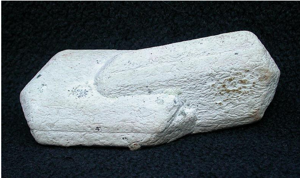
Image 13: A “Pig Egg” , Orthoclase converting to Kaolinite (Pseudomorph Kaolinite after Orthoclase). Specimen is from Goonbarrow China Clay Pit, Cornwall, England, UK .
