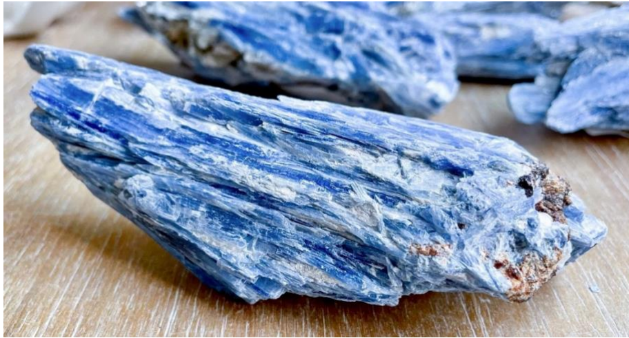
IMAGE 7: Some consider Kyanite to be fibrous while others describe it's fracture as splintery.
