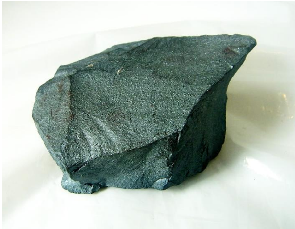
IMAGE 12: Another sample of Specularite showing sub-conchoidal fractures.
