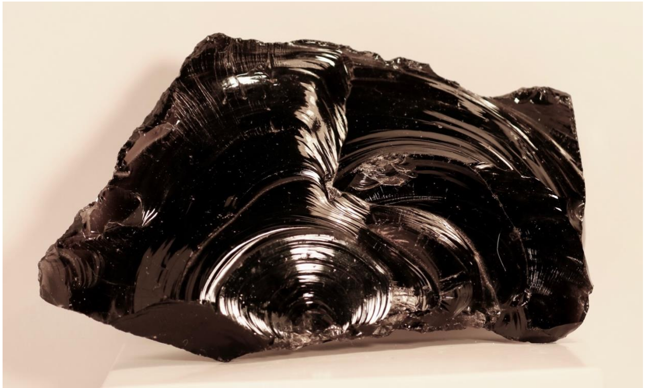
IMAGE 2: Black obsidian exhibiting classic conchoidal fracture. Note the concave and convex surfaces with scalloped patterns. Photo by T. Jeffries
