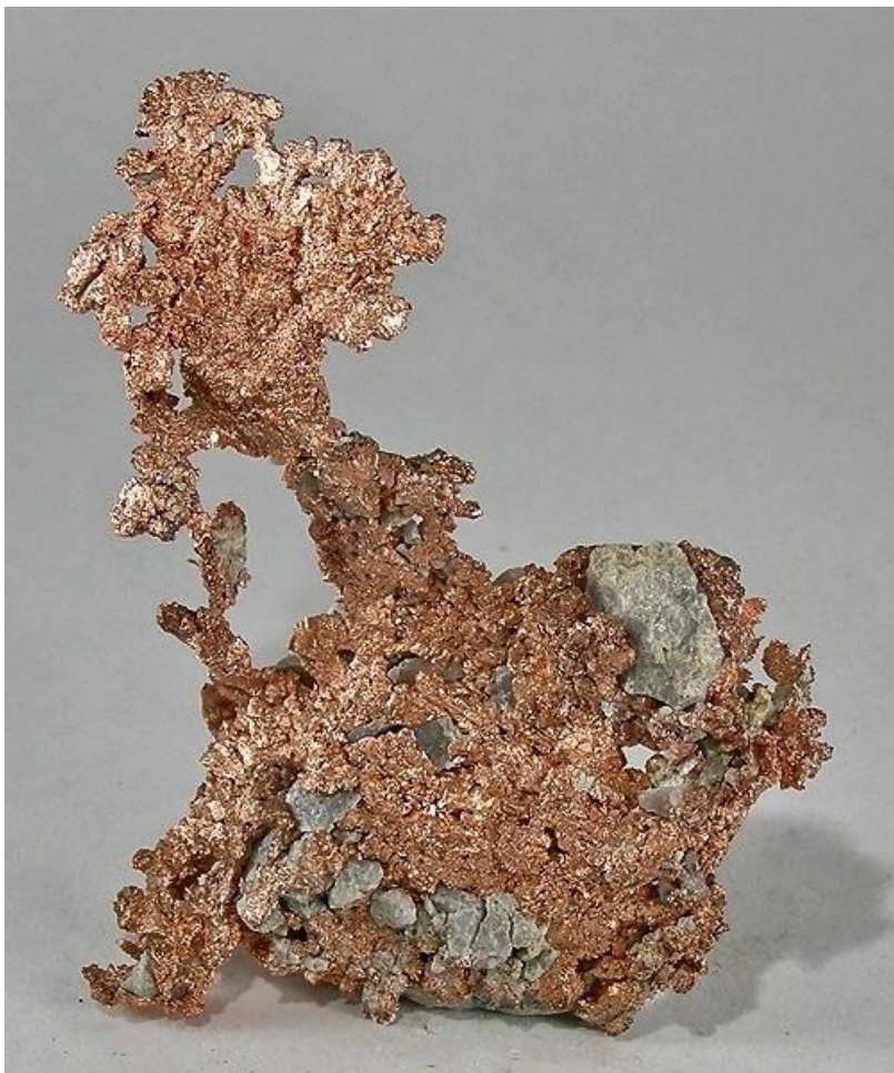
IMAGE 8: A specimen of native Copper showing the rough, jagged, and sharp surfaces associated with a hackly fracture. Autorius Rob Lavinsky, iRocks.com – CC-BY-SA-3.0, CC BY-SA 3.0,
