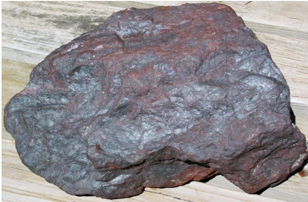
IMAGE 11: Specularite variety of Hematite (high-grade iron ore) from Minnesota. Note the irregular/uneven fracture pattern. Photo by John St. John
