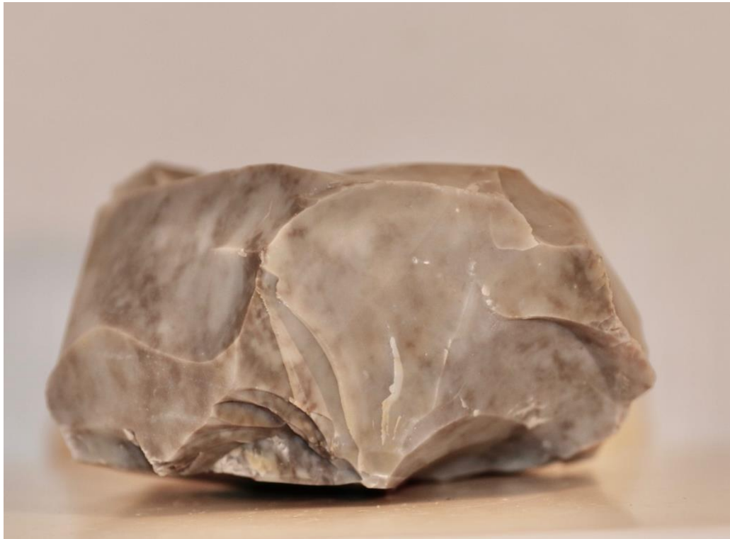
IMAGE 4: Flint from Flint Ridge, Ohio showing sub-conchoidal fracture. Note the shallow and less pronounced concave and convex surfaces. Photo by T. Jeffries
