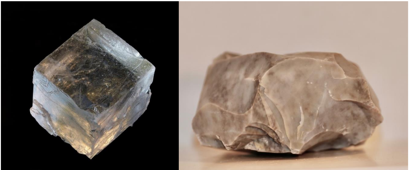
IMAGE 1: The Calcite on the left shows 3 planes of cleavage. Note the flat, smooth surfaces where the mineral 'cleaved' along planes of weakness. The Flint on the right demonstrates sub-conchoidal fracture. Note the surfaces are not flat and are randomly formed on the surface.
