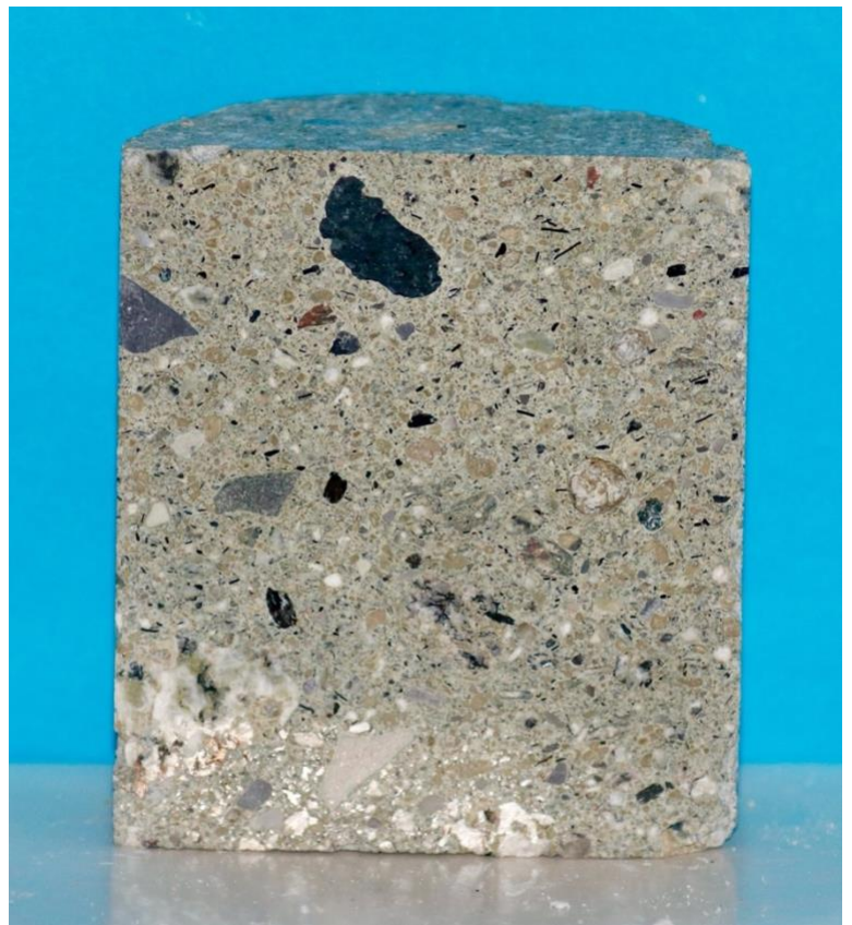
IMAGE 13: This is part of a core sample taken from the Victor Diamond Mine in Ontario, Canada. It is a nice example of an ultra-mafic Tuff, observe the greenish tint. The rock is Kimberlite, a common source of Diamonds. Note that Kimberlites are a complex group of rocks and not all Kimberlites are Tuffs. There is an ultra-mafic bluish Laprolite Tuff (similar to Kimberlite) found at the Crater of Diamonds State Park, Arkansas. Photo by Tracie J.
