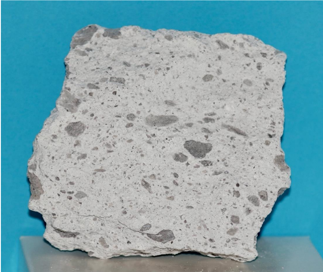
IMAGE 6: This is a sample of Bishop Tuff collected near Mammoth, California. This is a good example of an ignimbrite/ash-flow Tuff. The hot ash (light gray) and pumice clasts (dark gray, angular fragments) welded together when they fell. So we could use modifiers such as: felsic, Rhyolitic, ignimbrite/ash-flow, welded, and vitric-crystal (it is mostly vitric with some mineral crystals such as biotite, quartz, and plagioclase). Photo by Tracie J.
