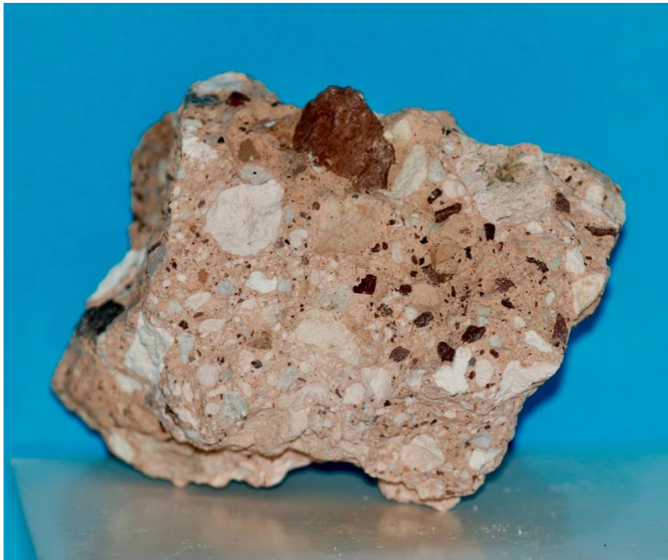
IMAGE 11: This is an example of a Tuff Breccia with a lot of interesting traits. It has numerous angular clasts. The white clasts are Pumice and the darker clasts originated from the walls of the volcanic vent. Hence, it is a vitric-lithic Tuff. It can also be described as felsic, Rhyolitic, and welded. This is a good example of the term 'Tuff' being used in a broad context. This sample is obviously not 75 % or more ash. It was collected in the Last Chance Canyon area in Kern County, California. Photo by Tracie J.
