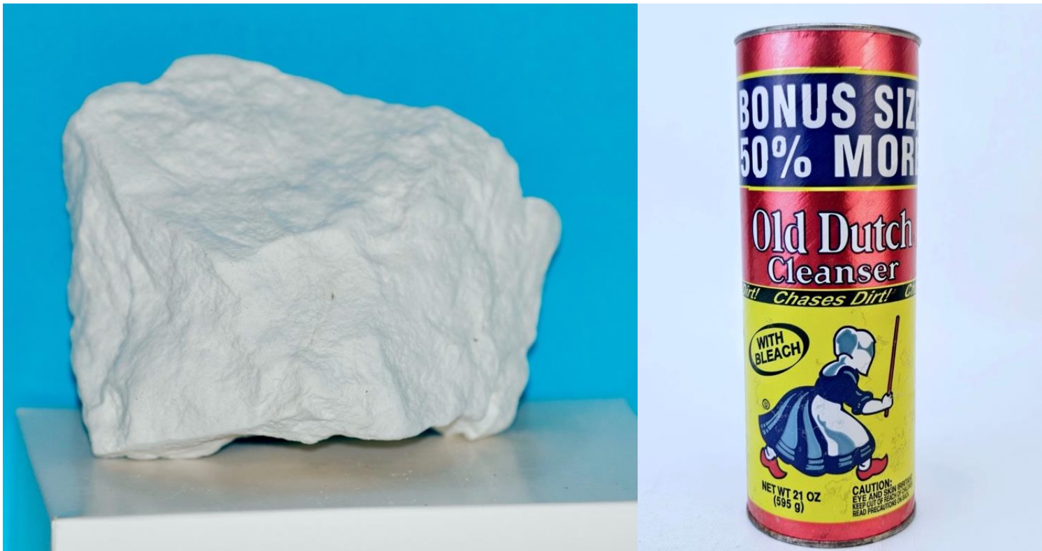
IMAGE 4 and 5: This is a sample of pure Tuff, it is 100% ash. This Tuff can be described as felsic, Rhyolitic, vitric, (Pumice based), ash-fall, non-welded, and loosely lithified. It is very light-weight, porous, and soft. It was collected from Cudahy Mine, in Last Chance Canyon, California. During the early 1900's this material was mined for 'Old Dutch Cleaner', an abrasive cleaner similar to Ajax, and Bon Ami. Image by Tracie J.
