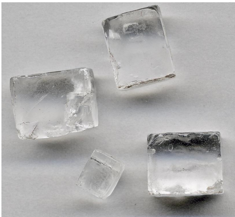
IMAGE 11: Cleaved cubes of Halite (salt) showing three cleavage planes at 90^\circ . Halite and Galena are unique in that their cleaved form is also their crystal form.
