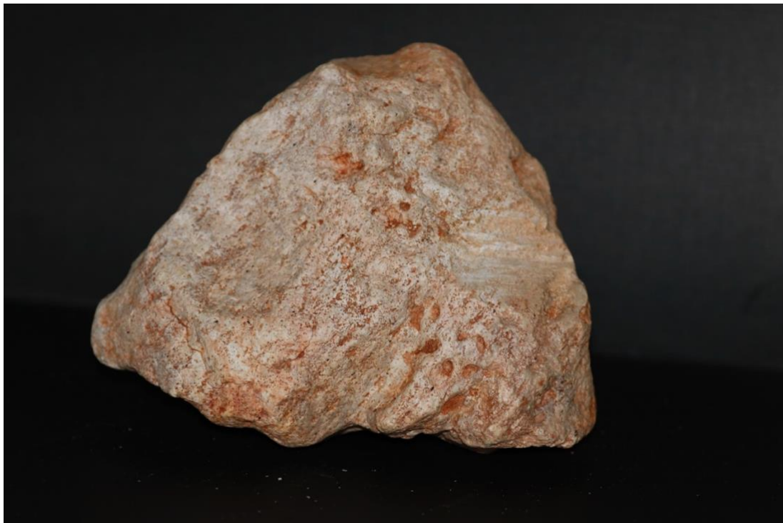
IMAGE 6: This is an example of Soapstone. The rock is fine-grained, non-foliated, and feels slippery or 'soapy' to the touch. This Soapstone was collected in Catawba County, NC. This sample is approximately 14 x 11 x 5 cm in size. Photo by Tracie J.
